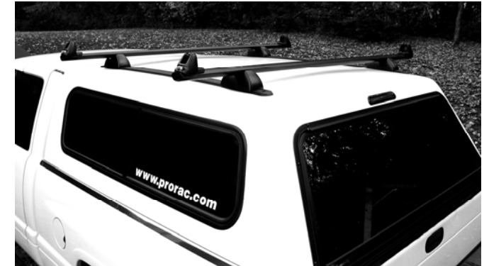
Photo shown with optional sliding load stops and 72" load bars.
