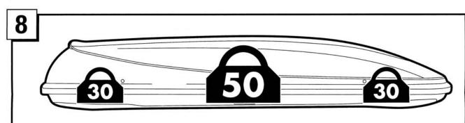
Make sure that loads are evenly distributed inside the roof box. Do not exceed the maximum permitted load of 110 lbs./50kg. for the box or the
