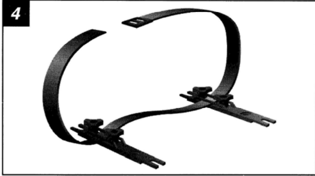
4. Insert the straps through the eyes of the brackets. Loads must be secured with the help of straps to prevent them from sliding, and fastenings should be checked at regular intervals.
