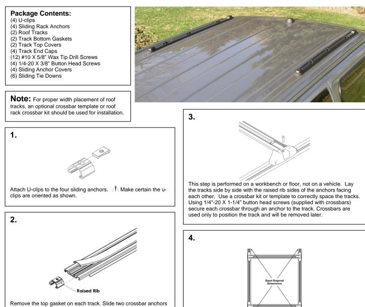
onto each track. The sides marked with the raised ribs should face each other.
